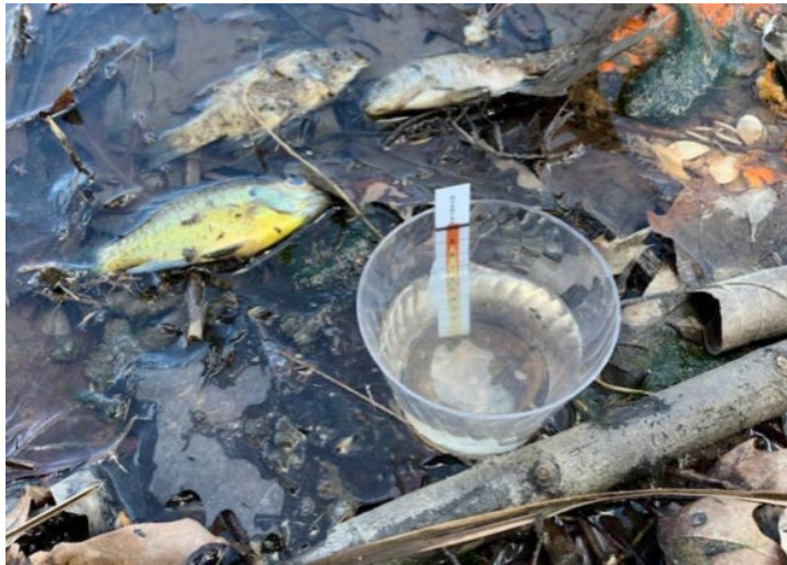
Fish kill in Lake Varuna, Gaithersburg, MD due to high chloride, Source: Karl Van Neste / Muddy Branch Alliance
