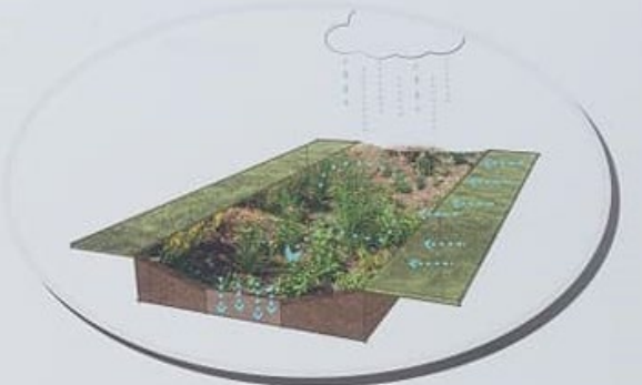
Bioswale rendering courtesy of Rutgers Water Resources Program Green Infrastructure Guidance Manual
